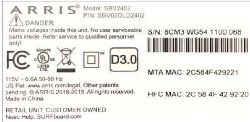
The telephony modem label is located on the bottom of your SBV2402. It contains the specific telephony modem information that you may need when contacting your service provider or [ARRIS technical support](#) (page 12).
